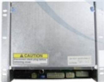
DIXIE NARCO SIID CONTROLLER BOARD
